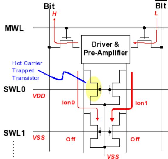
Figure 4. Reading the Bit Cell
