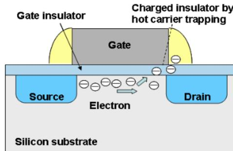
Figure 1. Hot Carrier Trapping
