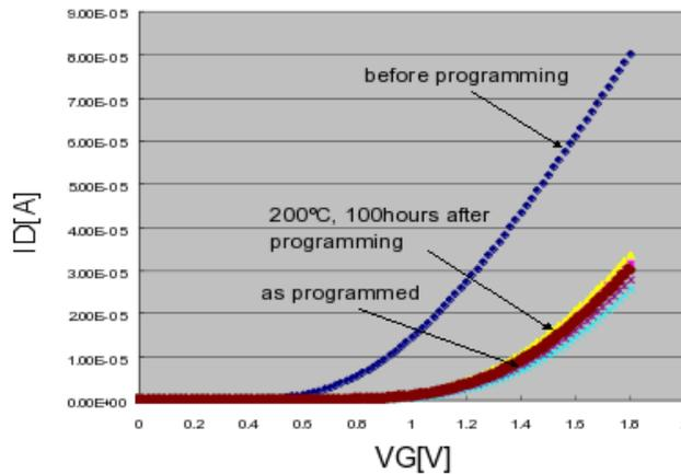
Figure 2.  $I_d$ - $V_g$  Curve for Unprogrammed and Programmed Bit Cell
