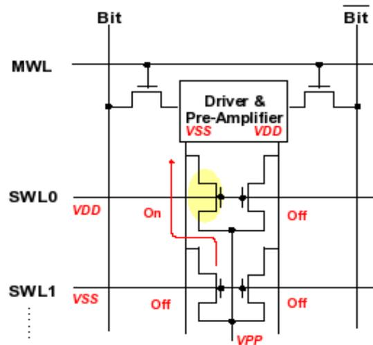
Figure 3. Programming the Bit Cell
